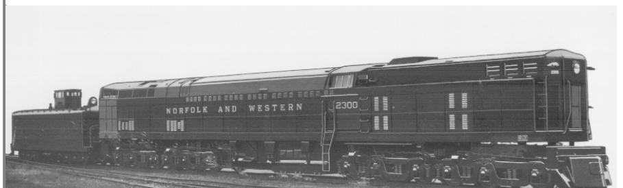
N&W Coal Fired, Steam Turbine, Electric Drive Locomotive #2300 - "Jawn Henry" Photo courtesy Roanoke Chapter NRHS
